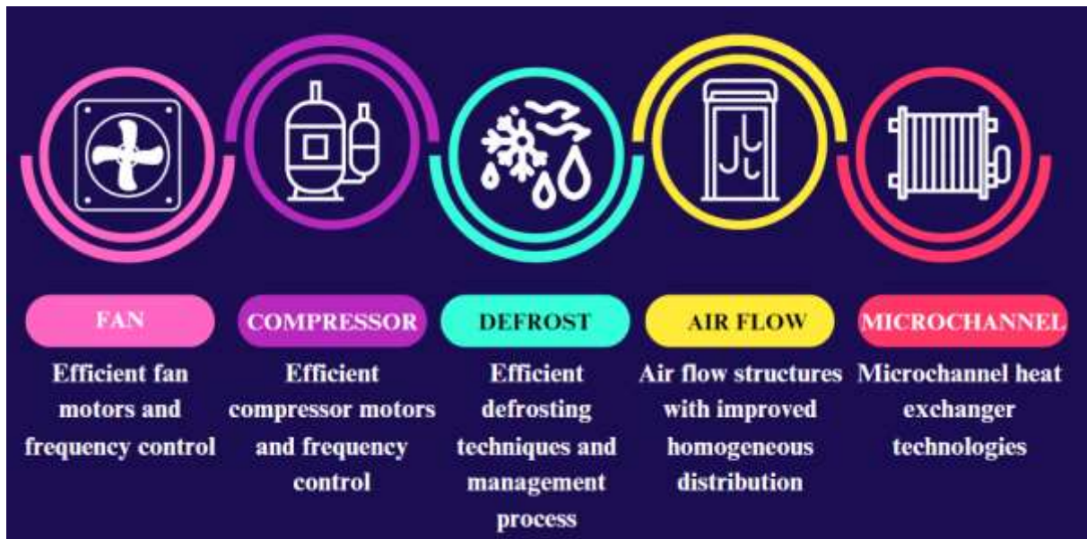
Figure 1. Examples of new or emerging technologies in cooling systems
