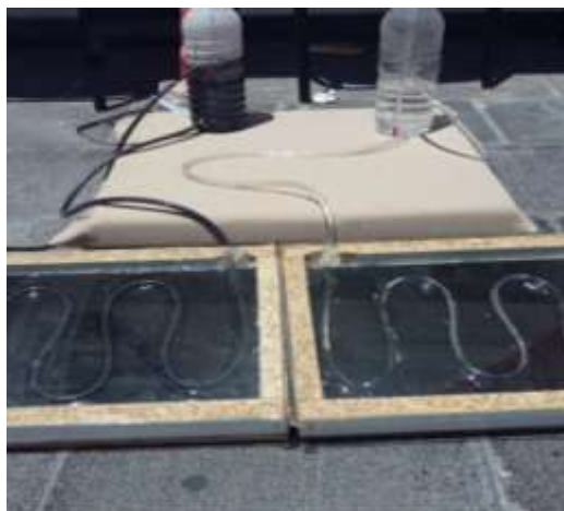
Figure 1. Prototype view of solar and Connection of solar collectors to the tank.
