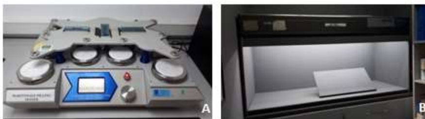
Figure 4. Martindale abrasion and pilling tester (A), Verivide CAC150 light cabinet (B)
