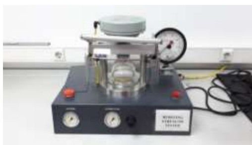
Figure 2. Messmer Buchel burst strength test device used in the experimental study
