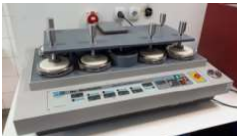
Figure 3. Martindale abrasion and pilling test device used in the experimental study
